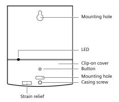
Mark the positions of the two drill holes on the wall. Drill two holes suitable for 6 mm wall plugs. Screw the upper screw into the wall plug and mount the casing by fixing the upper mounting hole onto the screw. Screw the casing into place using the lower mounting hole.
